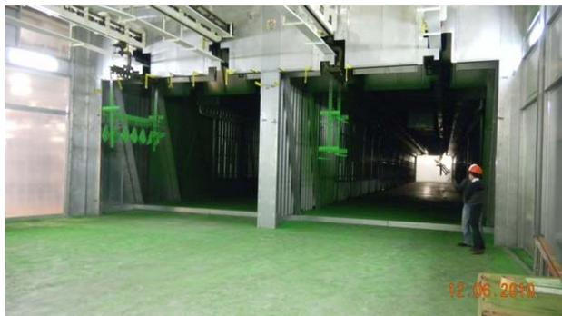
Curing Oven at 400°F – Seal Technology prevents migration of hot oven air into the plant. - 2010
